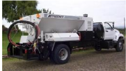
A Jetpatcher mounted on a truck chassis
